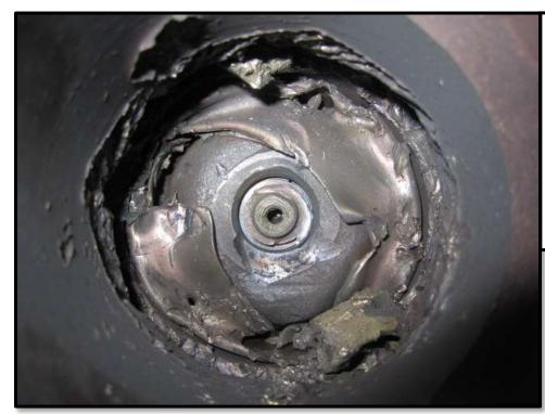
This is the result of a successful turbine burst containment test. Note large chunks of wheel embedded in housing, and torn sheet metal heat shroud. Despite internal damage, exterior walls of the housing have remained intact.
