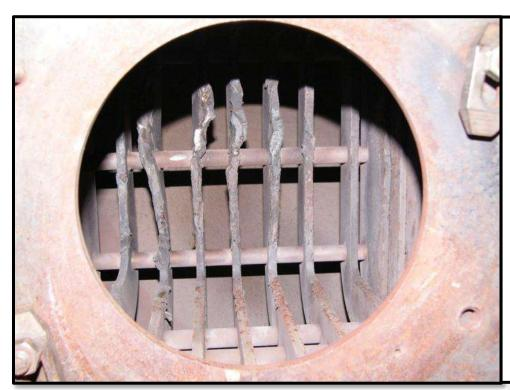
This grating is made of thick steel bars and is known as the "bug catcher." It is placed behind the turbine housing for Garrett® burst containment tests, to catch turbine wheels that may be ejected from their housings. This type of grating may be overkill on a racing vehicle, but it illustrates the need for some type of structure to impede turbine wheels from escaping through the housing outlet.
