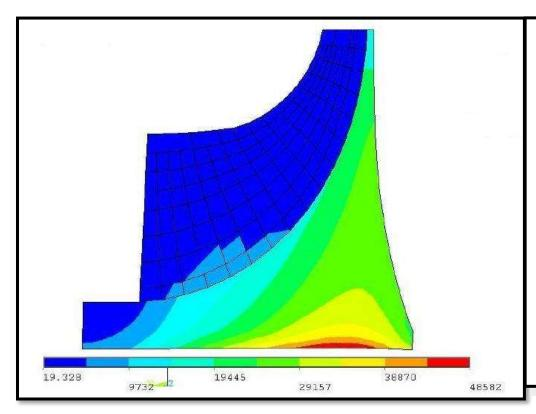
Stress concentration in a compressor wheel running at full speed, shown in half of a cross-sectional view. The distribution represents tangential (hoop) stress, which drives LCF failure. Highest stress region is represented in red and is at bottom right corner, which is at the thru-bore of the wheel, in line with the exducer diameter. Cracks that lead to hub burst will most likely start in this red region.
