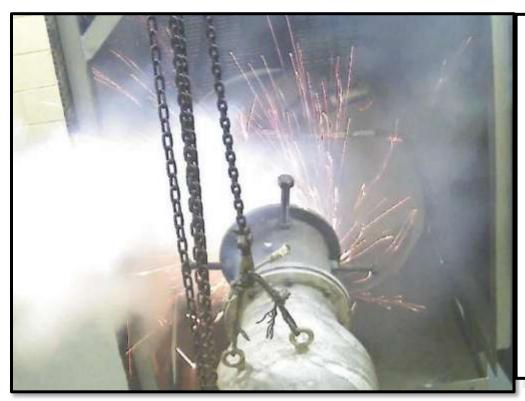
Burst containment testing can get exciting! This still image was taken from video of a Garrett® GTX3076R compressor housing containment test. The turbocharger is barely visible behind the cloud of sparks; the object in the foreground is the turbine outlet pipe that collects the exhaust gases. After the compressor wheel burst, the turbine wheel contacted the turbine housing, causing the sparks.
